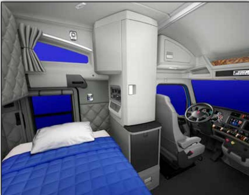
*For lower-profile and weight-sensitive applications, the Kenworth W990 with a 76-inch mid-roof sleeper reduces weight by 100 lbs over one of our full-height options. The spacious sleeper can be ordered with either the optional back wall storage system or folding upper bunk to meet your individual needs.*
