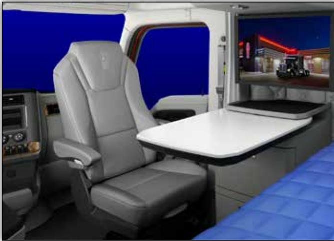
*The Driver's Studio includes the 180-degree swivel passenger seat and swivel table option set, which maximizes the driver's living space by combining the cab and sleeper into a large studio, allowing the driver to relax in comfort in the passenger seat rather than being confined only in the back of the sleeper.*
