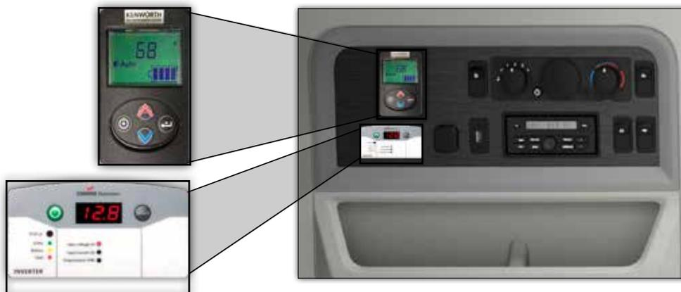
*The sleeper control panel is a convenient central location for all the items you need to control the sleeper environment, along with entertainment and interior lighting.*
