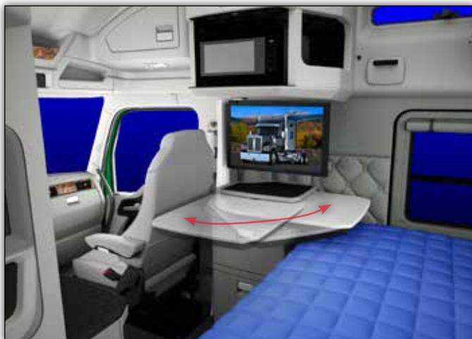
*To maximize stand-up room in the sleeper, a pull of the latch unlocks the table which may be rotated 90 degrees above the bunk, also giving you easy access to the drawers below.*
