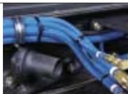
Kenworth offers wirebraid hose for its air brake systems – an extra that pays off in peace of mind when your application takes you miles from anywhere.
